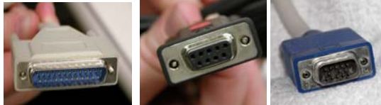
Parallel Cable (25 pin male (Printer)) Serial Cable (9 pin female) Video Cable (14 Pin male)
