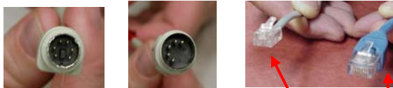
P/S 2 Connector Mouse/keyboard AT Connector Older keyboard RJ-11 Telephone (4 wires) RJ-45 Network (8 Wires)
